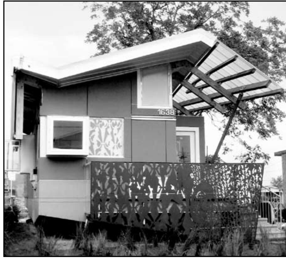
Morphosis Architects designed The FLOAT house, which is an affordable, flood-safe housing unit that will float with rising water.
